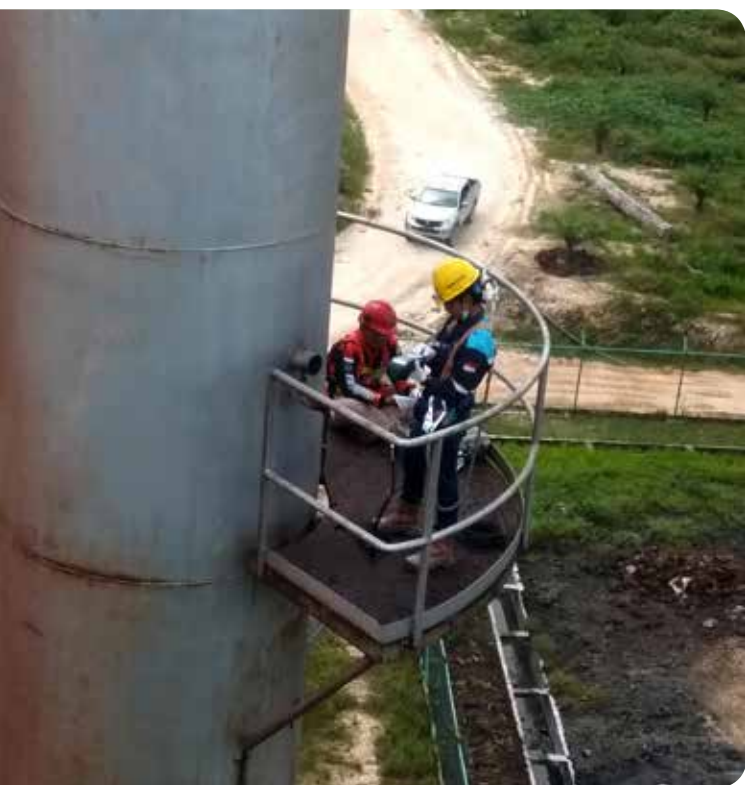
↑ Sampling emissions from a boiler chimney at PMP's palm oil mill.
