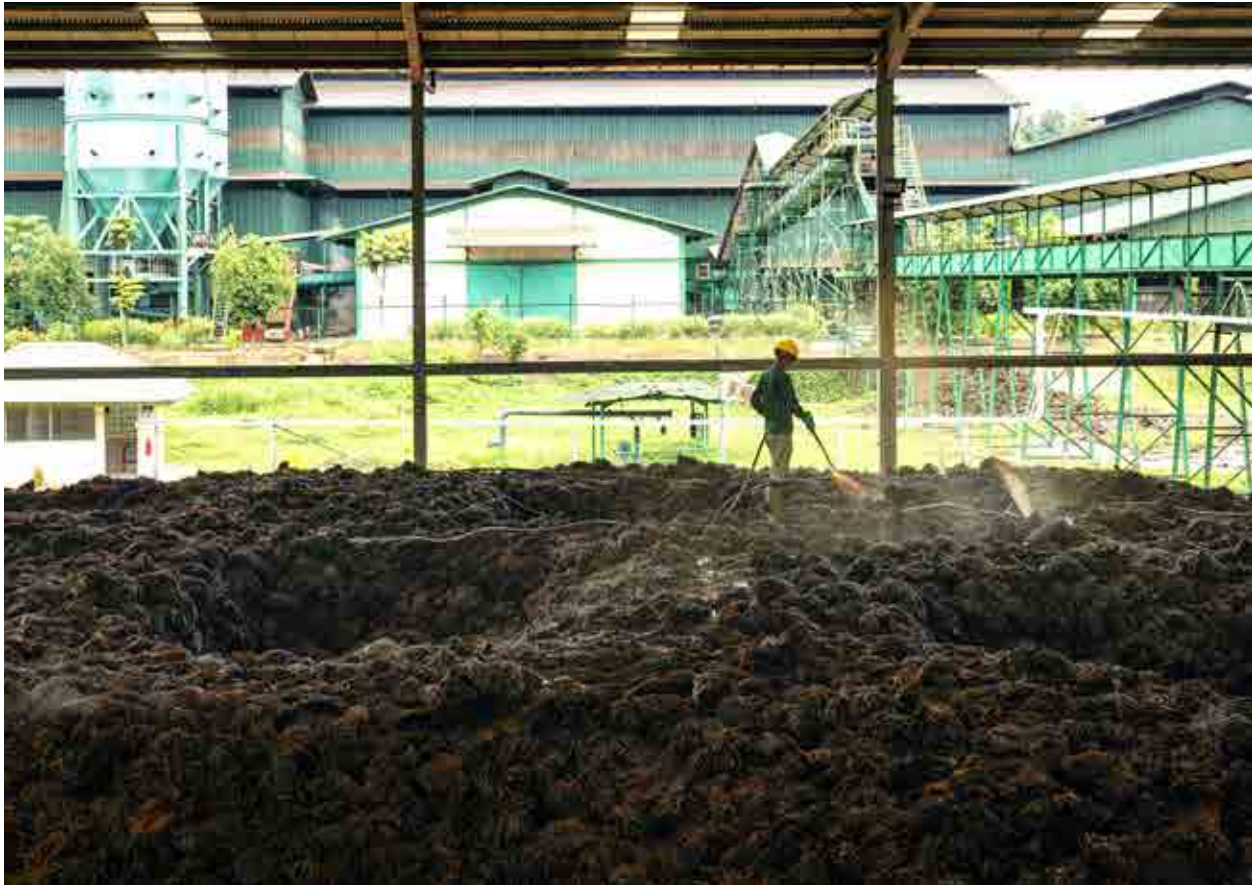
A Worker spraying POME onto empty fruit bunches to produce compost
