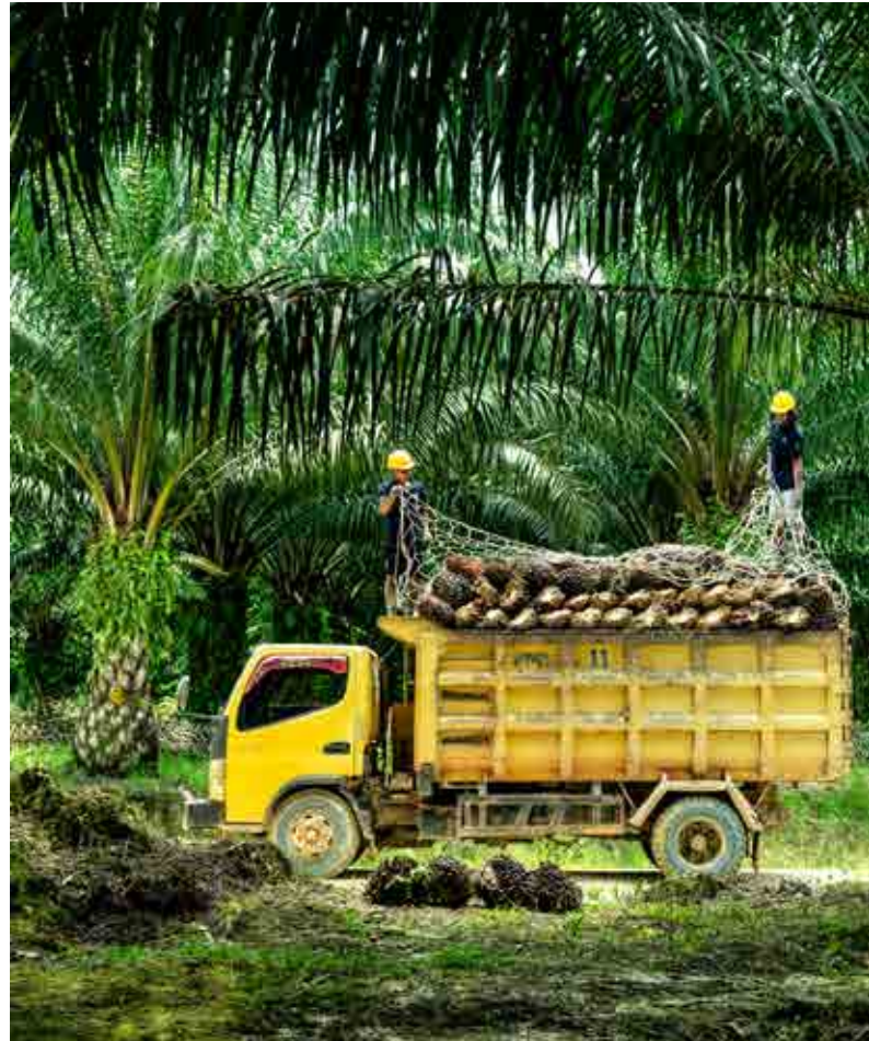
Setting up safety nets on FFB trucks helps prevent fruits from falling during transportation.
