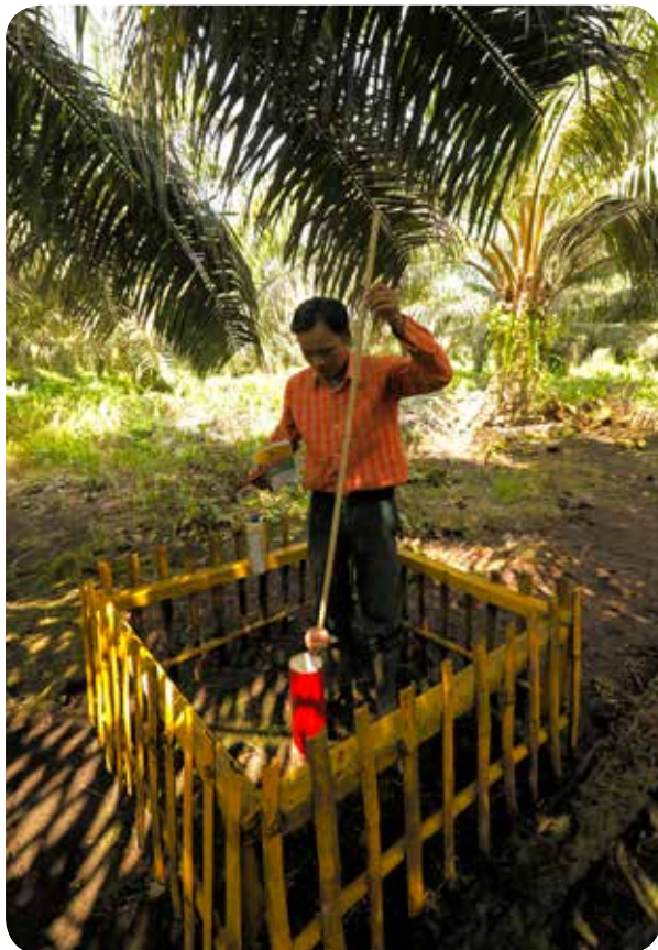
▲ Measuring water level in ANJAS using piezometer.
